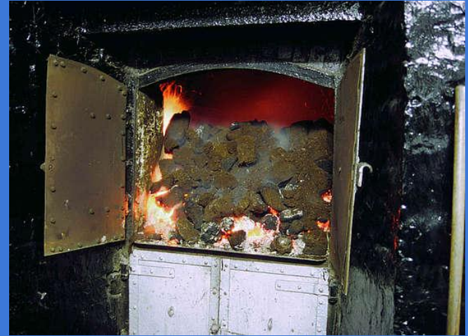
Peat-fired Kiln at Laphroaig Distillery
